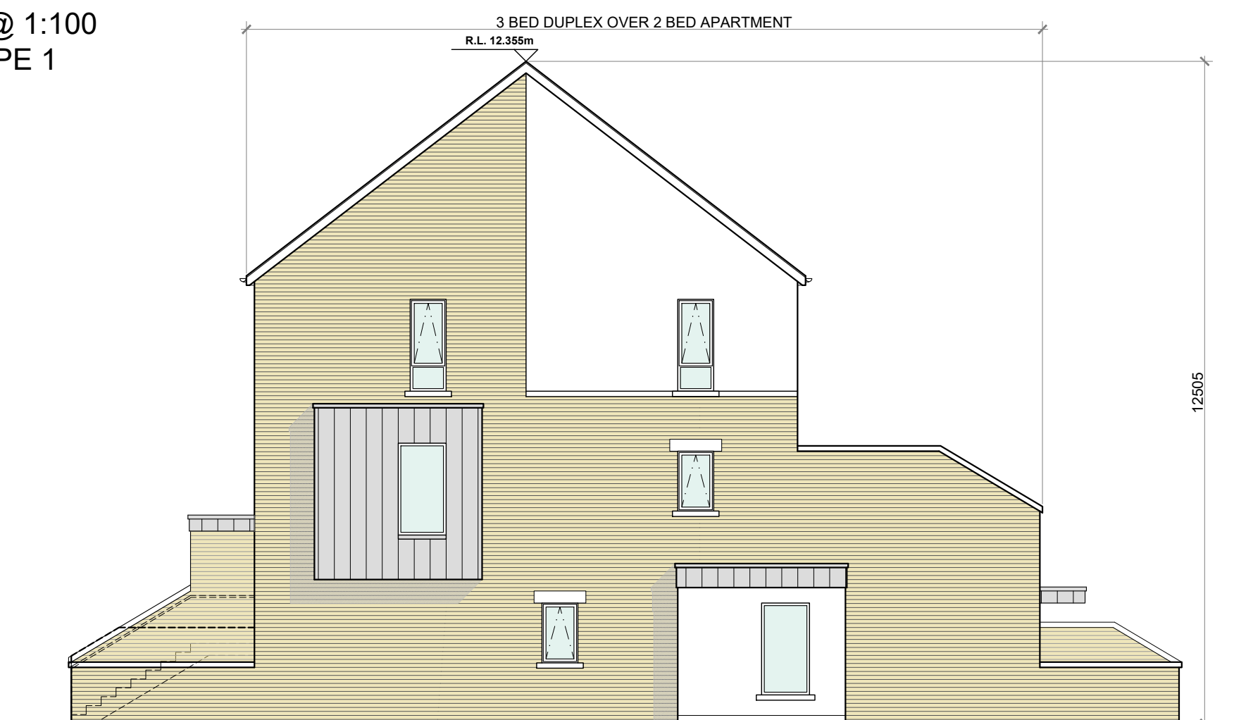
SIDE (DUAL FRONTAGE) ELEVATION @ 1:100 DUPLEX BLOCK TYPE 1
