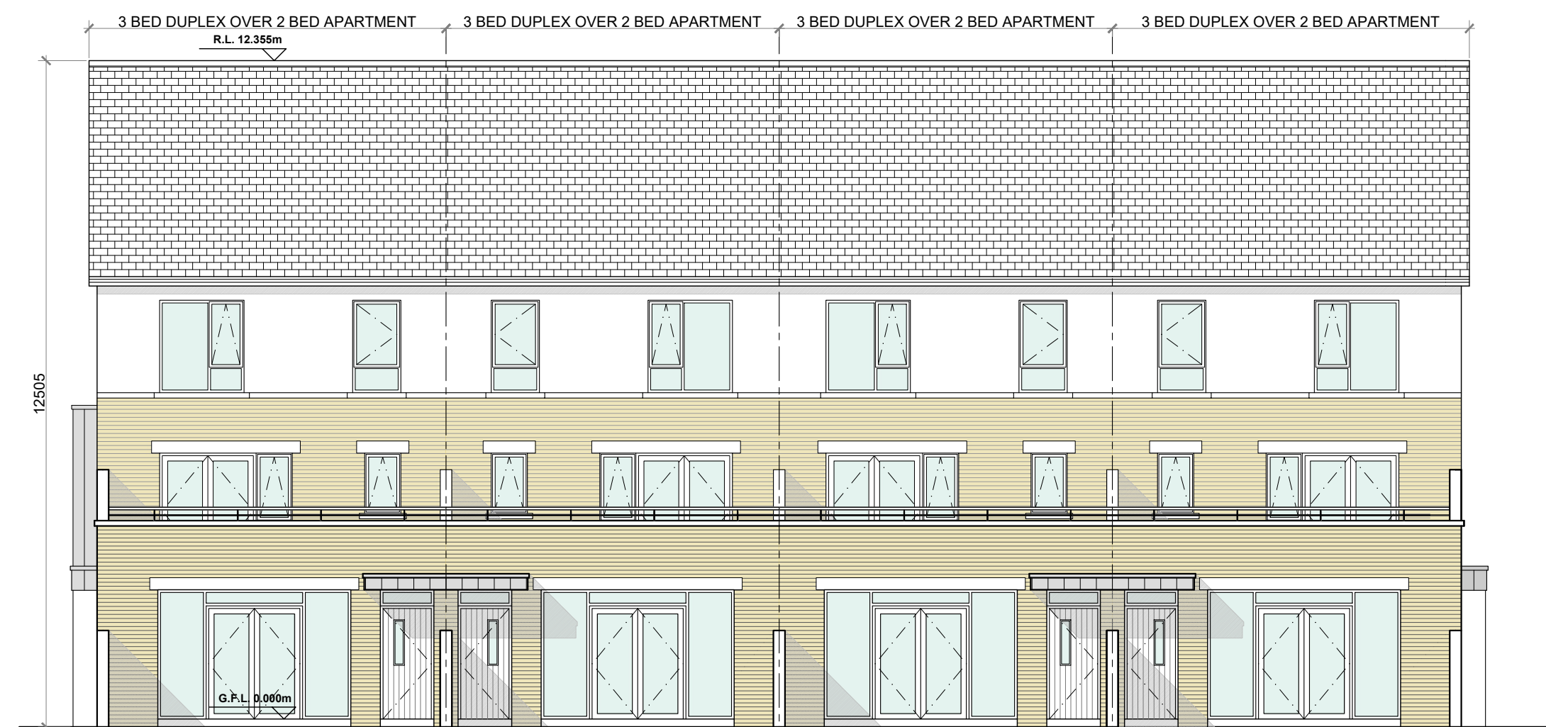
REAR ELEVATION @ 1:100 DUPLEX BLOCK TYPE 1
